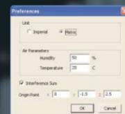
Enter the settings for the temperature and humidity of the air (Air Parameters), the phase interference (Interference Sum), and the coordinates of the person speaking or performing (Origin Point).
