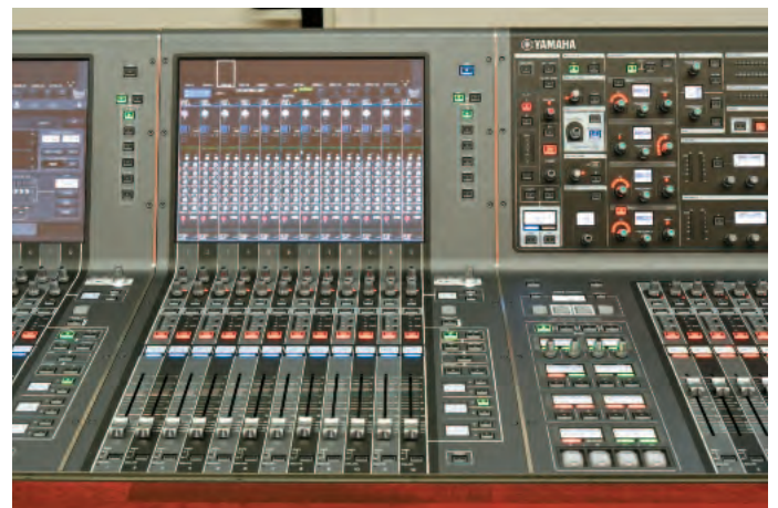
One of three 12-channel fader bays on the PM10 console's interface; the channel section can be seen in the top right of the picture
