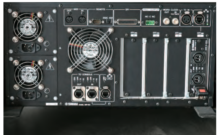
DSP engine from the front and rear. On the front side, there are two slots for cards in the familiar MY format. Up to four HY cards for TWINLANe or Dante cards can be used on the back. The HY cards can transmit up to 256 (TWINLANe) or 144 (Dante) channels. The DSP engine is of course equipped with two power supplies
