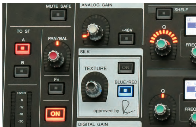
Silk setting with the selection "blue" for low-frequency and "red" for high-frequency as well as the texture setting for the intensity of the Silk processing
