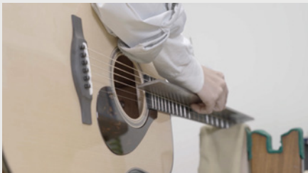
Inspecting the neck alignment
