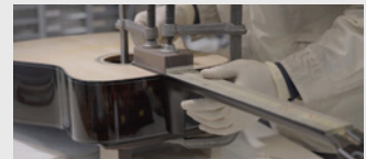
Attaching the fingerboard to the body
