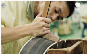
Final adjustments are made by hand, sanding to ensure a perfect fit.
