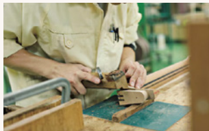
The process of repeating fine adjustments with a hand plane, then securing the neck in the correct position
