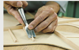
Bracing Shaping Process of L36
