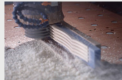
Bracing Shaping Process of FG9 (CNC Machining)
