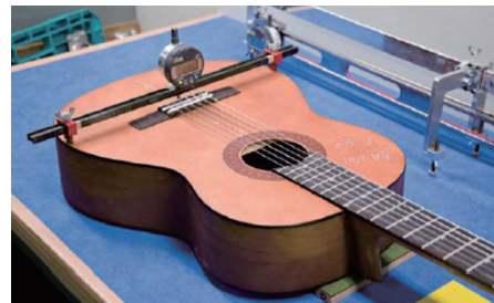
We check for any warps or distortions after the environmental test.
