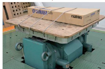
A guitar undergoing intense vibration testing to simulate truck transportation conditions
