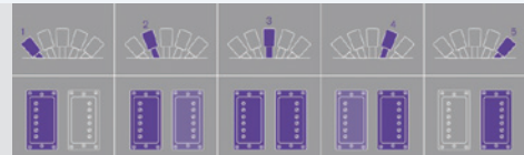
Pickup Operation by Selector Position. Light shading indicates phase shift via "Half Phase Out."
