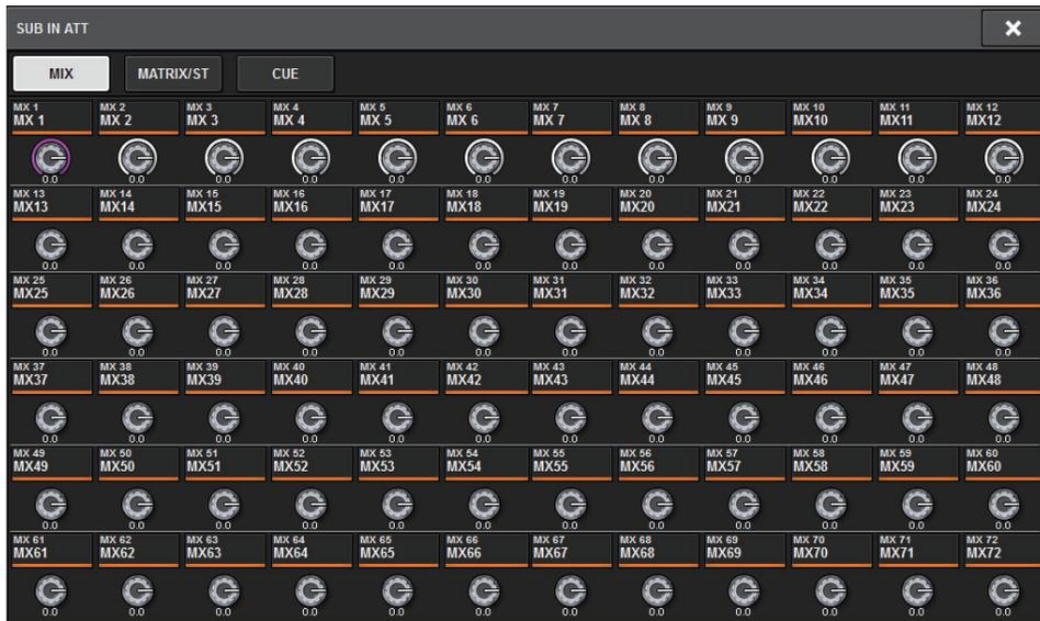
Press one of the tabs to select the output channel type, and then use the knobs to adjust the gain for each channel.
