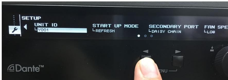
2. Rotate the encoder until the desired ID number is shown. It can be in the range “Y000” to “Y07F”.
