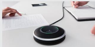
In a room with strong reverberation, cut the low frequency factor from the sound picked up by the microphone
