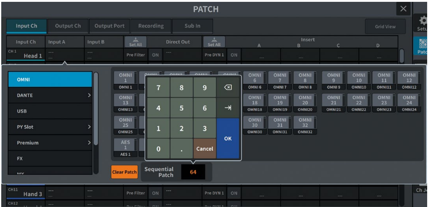
Sequential patching allows, for example, 64 channels to be patched in a single operation
