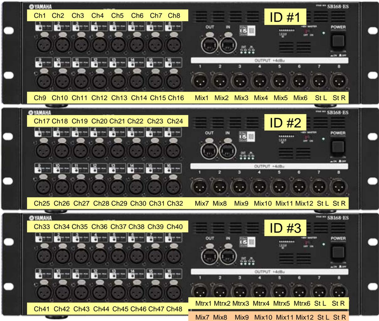
In Ring mode, there are only 16 available output channels in EtherSound network. So ID #3 box outputs copies ID #2 box as shown in orange box.
