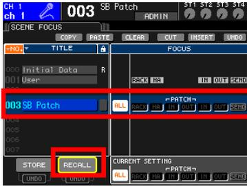
10. Recall the SB168 patch SCENE. (This recalls the IN and OUT patches.)
