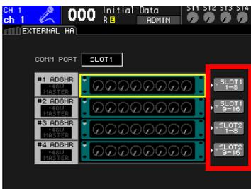
7. Open the Rack page and go to the External HA screen. Use the External HA Port Select button to assign all the displayed HA controllers to the slots. (This setup is not part of SCENE MEMORY and is set for all SCENEs.)
