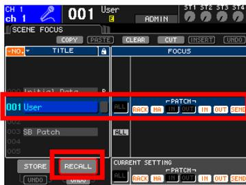
11. Recall the SCENE needing the SB168 patch. (IN and OUT patches are not recalled because of focus, the SB168 patches is used.)
