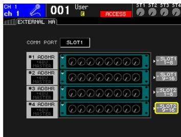
Using the PORT SELECT buttons, select the input ports to which the external HA (SB168-ES) is connected in groups of 8 channels.
