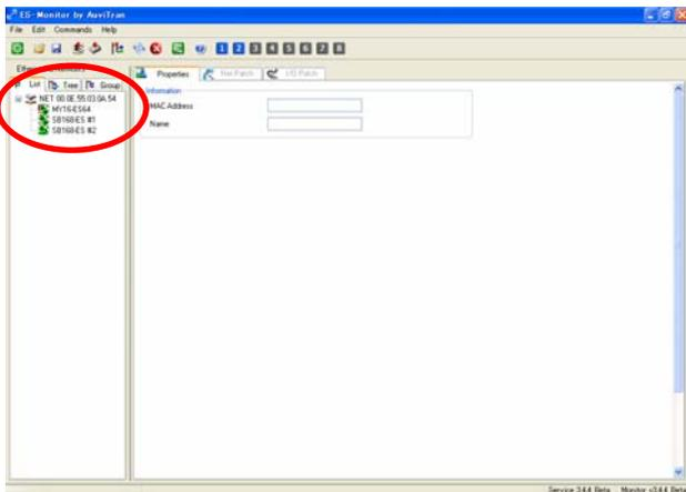
Devices being connected on a EtherSound network will be displayed on the “List” view.
