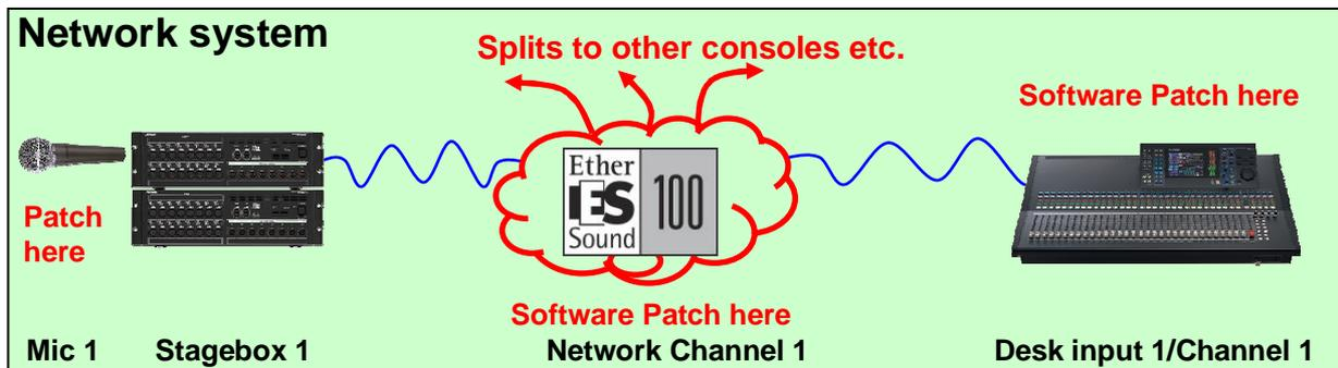
**Use the AVS-ESMonitor Quick Setup feature** to achieve network patching in one easy step. After it is set your system can work just like the traditional digital system, no further network patching is necessary, unless you redesign the system. However, the addition of a network to your setup prepares you for future upgrades of your signal path.
