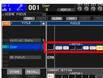
9. In the SCENE requiring the SB168 patch, change focus from [ALL] to [RACK] [HA] ..... [IN] [OUT] [With Send].
