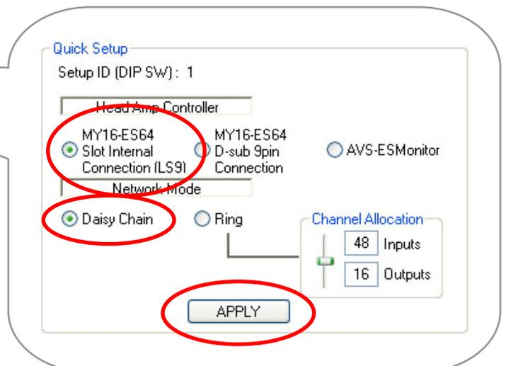
After the confirm box is checked all the network patching is done. HA control routing is setup and all information is saved to the EtherSound devices so they will remember after AVS-ESMonitor is disconnected or the power is cycled.
