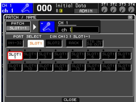
Port 1 of SLOT1 has been assigned to Input channel 1. Assign other slot inports as shown below using the same way.
