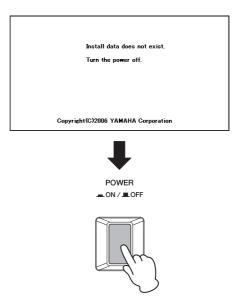
Turn off the DDK-7 and disconnect the USB flash memory device.
