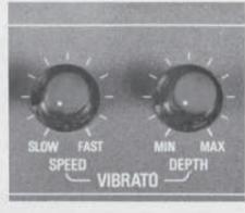
Note: The rate of "wah-wah" included in tones of "funny" and "wah guitar" as a preset part of the voice, can be altered using the vibrato controls. Place the vibrato lever (3) to "control" position, set the vibrato depth control (section (5)) to the minimum (counterclockwise) position. You can now adjust the vibrato speed control to obtain the desired rate of wah without introducing a vibrato effect.
