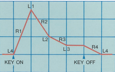
This waveform shows the eight parameters programmable in the envelope generators associated with each operator: Level 1 (L1) through Level 4 (L4), and Rate 1 (R1) through Rate 4 (R4).
