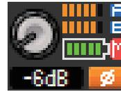
The RF level is shown for two channels (A and B).
