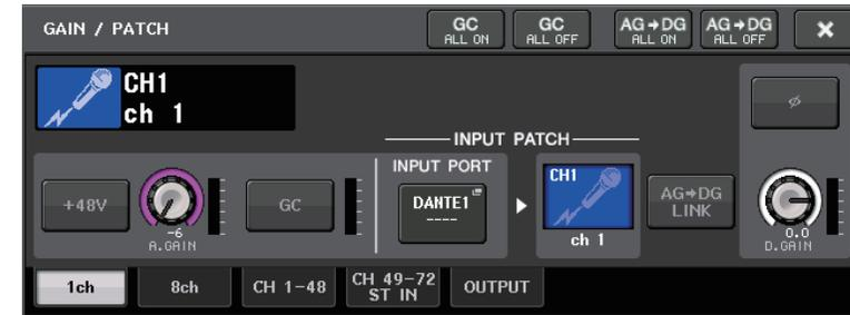
Press the INPUT PORT button, and on the PORT SELECT window select the port to which the output signal from the AXT400 is connected (OMNI 1).
