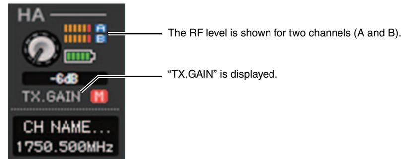
When the receiver is on and not connected via a ShowLink® remote control
