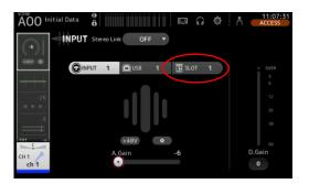
Input sources can also be set for multiple channels simultaneously. Open the menu screen on the INPUT screen by pressing the menu key, and select All SLOT to switch all the designated input sources at the same time.
