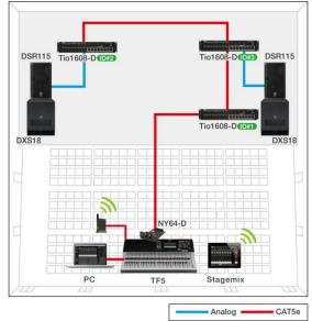
Stagebox system using the TF5 and three Tio1608-D racks
