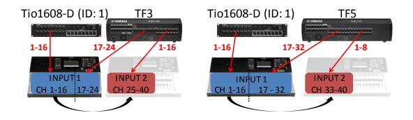
Input patching when using one Tio1608-D rack
