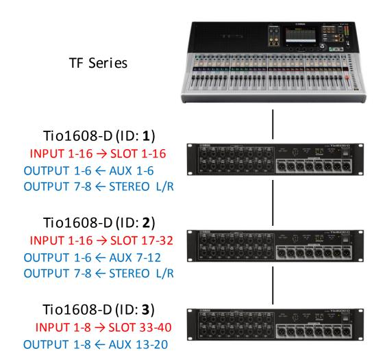
I/O patches on the Tio1608-D when using Quick Config
