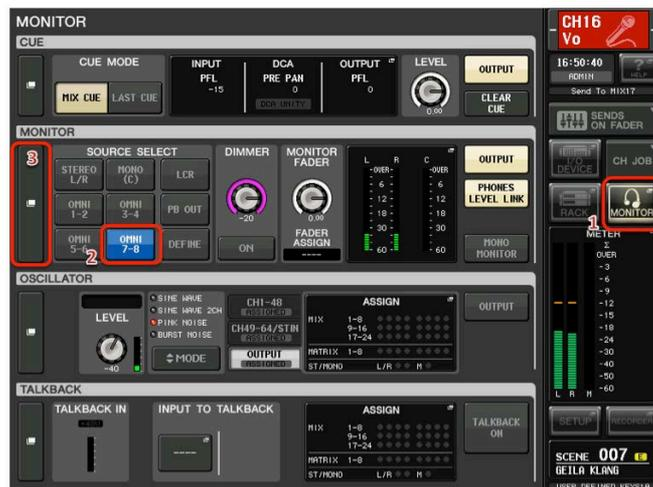
*[If the CL/QL mixer is in 5.1 SURROUND mode, there will be additional monitoring options, including external inputs via Dante. Use Dante Controller to route KLANG:fabrik's CUE output to 2 spare inputs of the CL/QL console. Then in the console's MONITOR menu, set "2CH MONITOR" as the SOURCE SELECT.*
