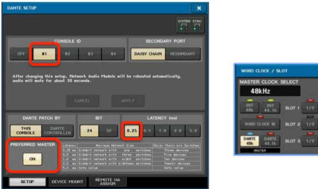
Because an in-ear monitoring system is being constructed, keeping the audio latency low is important. Make sure the monitor console has its latency set to 0.25ms. Then use only one network switch on stage between the R-series i/o racks, the monitor console and the IEM processor.
