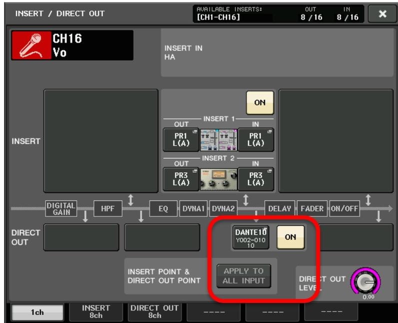
*[Note that the Stereo Input channels do not have a Direct Out function. So to send an Effect Return to KLANG:fabrik, use a pair of mono input channels instead.]*
