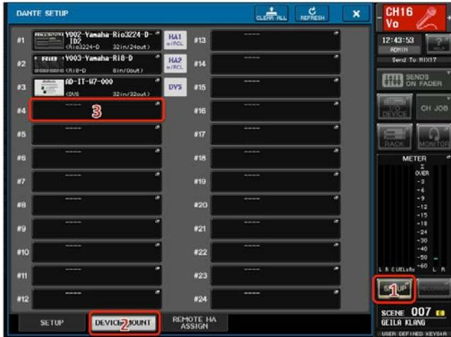
GO TO THE ONLINE DEVICE LIST, SELECT KLANG:fabrik and press OK. Then the device will appear as a mounted device. That will allow patching to be made from the console.
