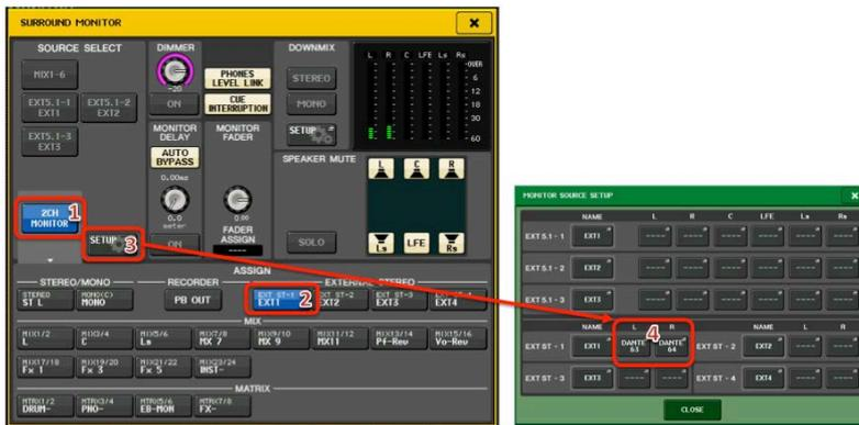
Open the MONITOR menu details to make sure “CUE INTERRUPTION” is enabled, and the MONITOR FADER is at a comfortable level. (The MONITOR FADER can also be assigned to a Custom Fader Layer). Set the MONITOR outputs to a suitable connection for the in-ear headphone amp or wireless transmitter. ONMI 7-8 outputs could be used if an analog connection is required.
